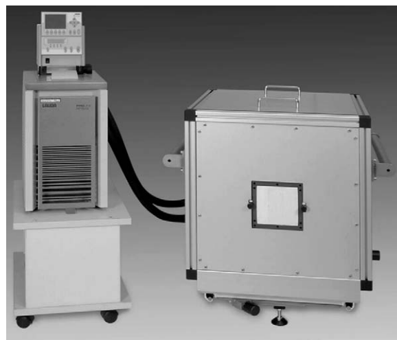
Fig. 2. Picture of the transportable water calorimeter with the corresponding cooling unit. The calorimeter has an almost cubic shape of about 60 cm edge length.
